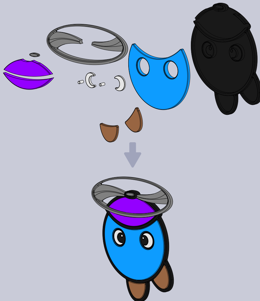
Recommended: Build parts at a 45° angle.
